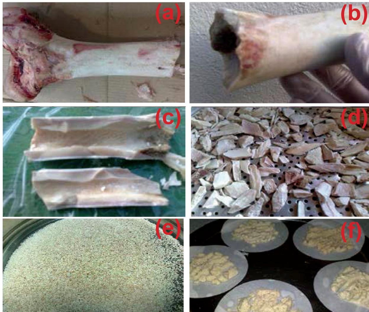
**Figure 1:** Bone powder preparation steps in order to extract hydroxyapatite: a) cutting, b) separation of soft tissue, c) removing of bone marrow, grinding d) first e) second (powder production) and f) prepared powders.
